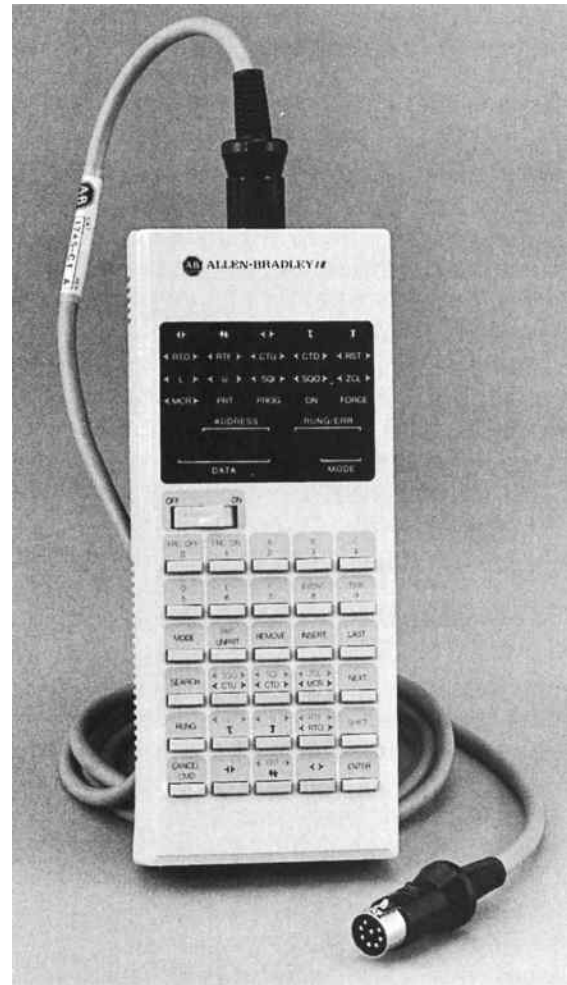
Fig. 58–11 Control logic can be entered into the processor from an operator program terminal. (Courtesy of Rockwell Automation)
