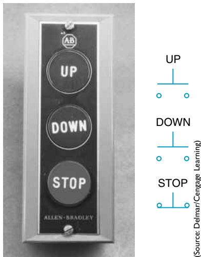
Fig. 6-1 Push-button control station with a general-purpose enclosure. The enclosure is usually made of molded plastic or sheet metal. This station contains three push buttons; two are normally open and one is normally closed.
