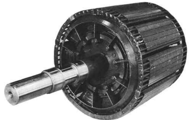
Fig. 39–1 Rotor of 300-hp, 720-rpm synchronous motor. (Courtesy of Electric Machinery Company, Inc.)
