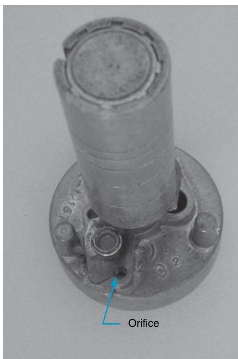
Fig. 3–23 The size of the orifice hole can be adjusted to change the time setting of the dashpot timer.
