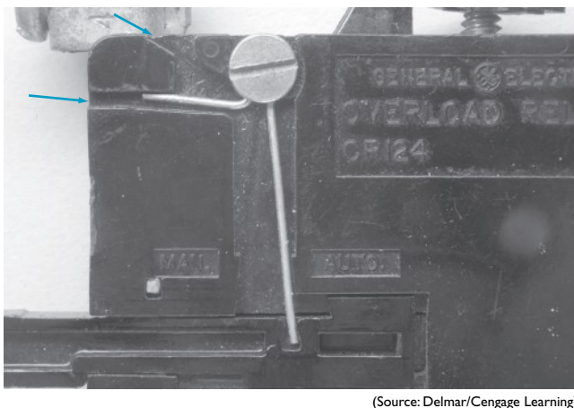
Fig. 3-18 The bimetal strip type overload relay can be set for manual or automatic reset by changing the position of the spring.
